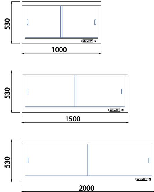
ARMOIRE SUSPENDUE AVEC MONOCOQUE ISOLEE AVEC POLYURETHANE ECOLOGIQUE A FAIBLE DENSITE, INTERIEUR ET EXTERIEUR EN ACIER INOXYDABLE, AVEC EVAPORATEUR STATIQUE AVEC DETENDEUR R404A, AVEC CONTROLE DE LA TEMPERATURE PAR UNITE ELECTRONIQUE, DEGIVRAGE A ARRET SIMPLE. TEMPERATURE D'EXERCICE +4/+16°C.
