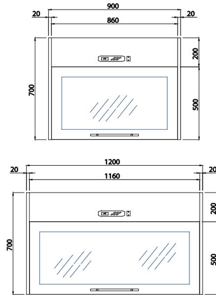
ARMOIRE SUSPENDUE AVEC COQUE ISOLEE AVEC POLYURETHANE ECOLOGIQUE A FAIBLE DENSITE. INTERIEUR ET EXTERIEUR EN ACIER INOXYDABLE AISI 304, SYSTEME AVEC DETENDEUR R404A; EVAPORATEUR LOGE SUR LE CHAPEAU ET EGOUTOIR EN INOX AVEC BAC DE AUTO-EVAPORATION DE L'EAU DE CONDENSATION SUR L'ARRIERE. TEMPERATURE D'EXERCICE +4°/+16°C.
