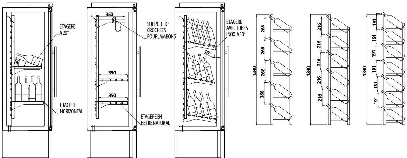
ARMOIRE REFRIGEREE VENTILEE AVEC COQUE EN INOX ISOLEE PAR POLYURETHANE ECOLOGIQUE A FAIBLE DENSITE, SYSTEME A DETENDEUR R404A AVEC DEGIVRAGE AUTOMETIQUE A ARRET SIMPLE, SOUBASSEMENT AVEC PIEDS REGLABLES, TABLEAU DE COMMANDE ELECTRIQUE FIXE DANS LA PARTIE HAUTE ET EVACUATION DE L'EAU DE CONDENSATION SUR LE FOND. TEMPERATURE D'EXERCICE +4°/+18°C.
