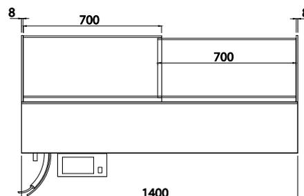
VITRINE REFRIGEREE VENTILEE CONÇUE POUR LE CENTRE D'UNE SALLE, AVEC SYSTEME DETENDEUR R404A, AVEC ELEMENT CHAUFFANT POUR CONTROLE DE TEMPERATURE ET HUMIDITE, AVEC UNITE DE COMMANDE ELECTRONIQUE FIXE SOUS, DEGIVRAGE A ARRÊT SIMPLE ET PLANS AMOVIBLES EN INOX. STRUCTURE SUPERIEURE COULISSANTE EN VERRE SUR PROFILS ANODISES ARGENT (ANODISES OR SUR DEMANDE), VERROUILLAGE AVEC CLE ET COTES EN VERRE FIXEES A FIL DE LA CUVE. TEMPERATURE D'EXERCICE +12°/+16°C.
