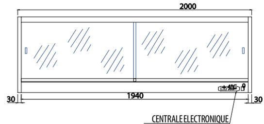
ARMOIRE SUSPENDUE AVEC MONOCOQUE ISOLEE AVEC POLYURETHANE ECOLOGIQUE A FAIBLE DENSITE, INTERIEUR ET EXTERIEUR EN ACIER INOXYDABLE AISI 304, AVEC EVAPORATEUR STATIQUE ET DETENDEUR R404A, TABLETTE EN VERRE OU BIEN EN INOX PERCE AVEC CONTROLE DE LA TEMPERATURE PAR UNITE ELECTRONIQUE, SORTIE DE TUYAUX EVAPORATEUR ET EVACUATION DE L'EAU SUR LE DOS, A DROITE. DEGIVRAGE A ARRET SIMPLE. TEMPERATURE D'EXERCICE +4/+8°C.
