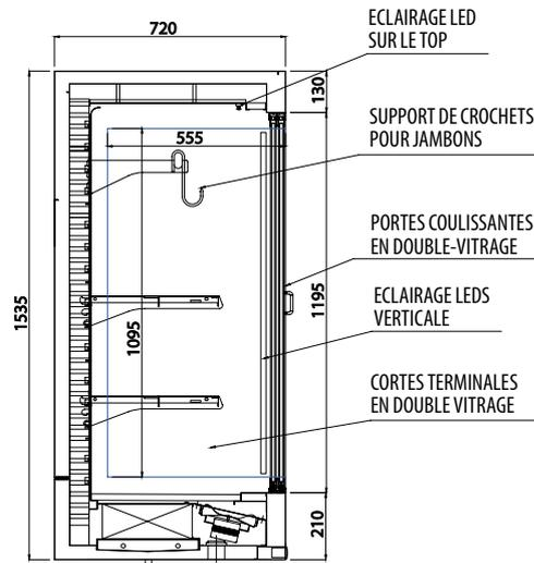
PRESENTOIR MURAL REFRIGEREE VENTILEE AVEC COQUE ISOLEE AVEC POLYURETHANE ECOLOGIQUE A FAIBLE DENSITE, INTERIEUR ET EXTERIEUR EN ACIER INOXYDABLE AISI 304, AVEC EVAPORATEUR VENTILE AVEC DETENDEUR R404A, CONTROLE DE LA TEMPERATURE PAR UNITE ELECTRONIQUE, DEGIVRAGE AUTOMATIQUE PAR RESISTANCES ELECTRIQUES. AVEC RIDEAU DE NUIT DEROLABLE, TABLETTES INTERMEDIAIRES REGLABLES EN INOX. AVEC TEMPERATURE D'EXERCICE +4/+8°C.
